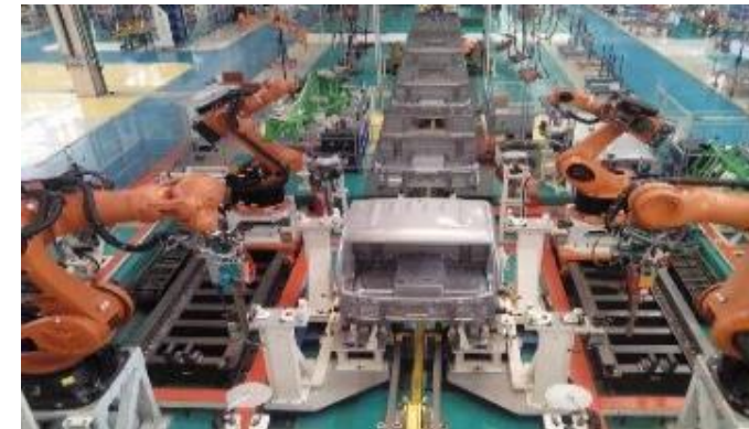
Robot in cab welding and press shop automation
